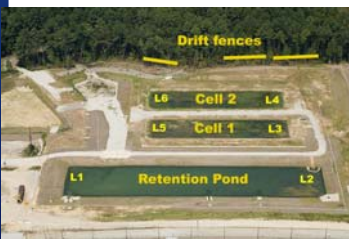
Figure 1. Sampling and experimental locations in the H-02 wetland complex. Effluent from industrial facilities and surface water runoff enters the retention pond near L2 and L3—the retention pond exhibits high concentrations of Cu and Zn. Water is piped from the retention pond to a splitter box on the east end of wetland cell 1, and flow is divided between the two cells. Water exits the system below L5 and L6, after a residence time of approximately 2 d. Amphibian sampling and experimental manipulations are conducted at locations L1 thru L6, which corresponds to a water chemistry gradient of decreasing metal concentration. Incoming adult amphibians and exiting juveniles are sampled at the drift fences on the north side.
